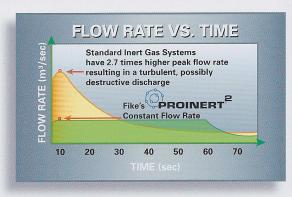
throughout the system. With **PROINERT**<sup>2</sup>, you can use small-diameter, low-pressure piping from the container to the nozzle – lowering your system costs.
